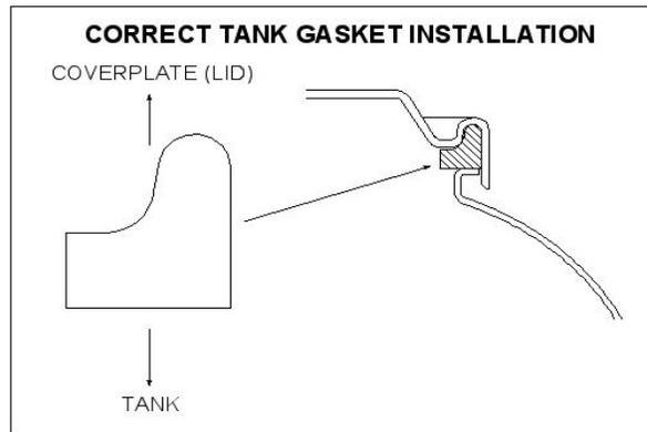
**E. The tank clamps are incorrectly adjusted.** Over time, the clamps can stretch and not seal the power head tightly to the tank. They can also get too tight and not close completely if the tank gasket is installed incorrectly. Please read FTN-017 ("Fixing tank clamp problems") for several suggestions to solve these issues.
